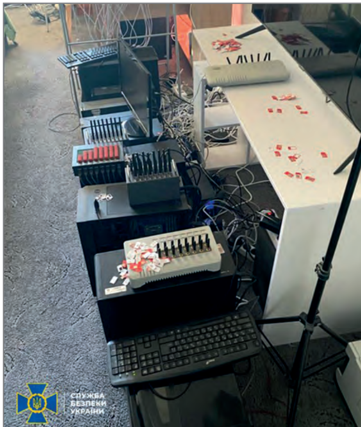
Figure 15. SMS/GSM gateway and SIM Card Batches Confiscated by Ukrainian Law Enforcement
